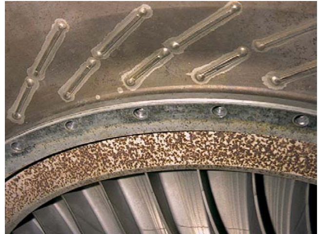
Figure 3-22. Hot Corrosion on Engine Components
