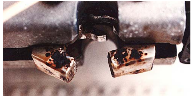
Figure 3-28. Failed Chromium Plate
