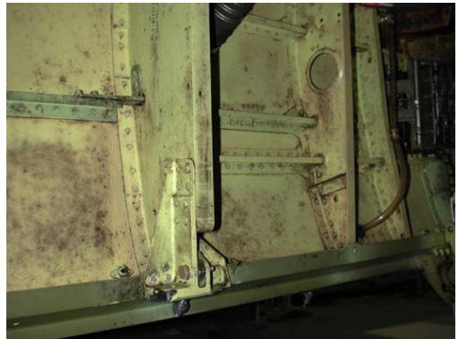
Figure 3-30. Biological Growth on Helicopter Wall
