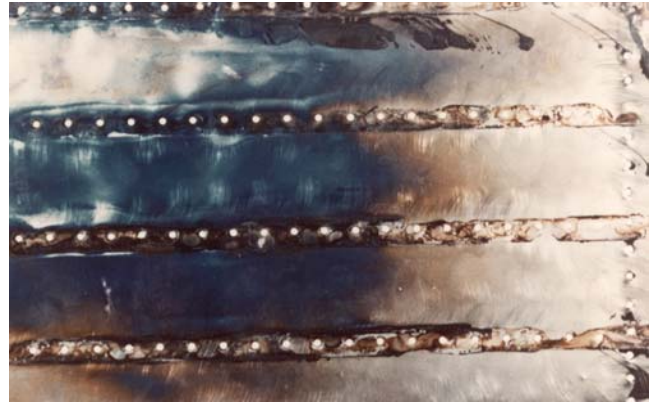
Figure 3-26. Color Changes in Titanium Due to Heating
